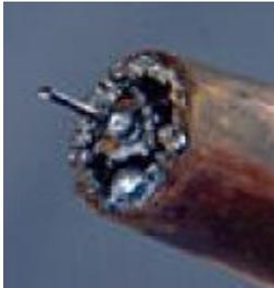
Wire drag, caused by poor wire feed. Lube-Matic pads and liquid help keep liners free of unwanted build-up and deposits inside the liner that cause wire drag. The result as shown above is an
